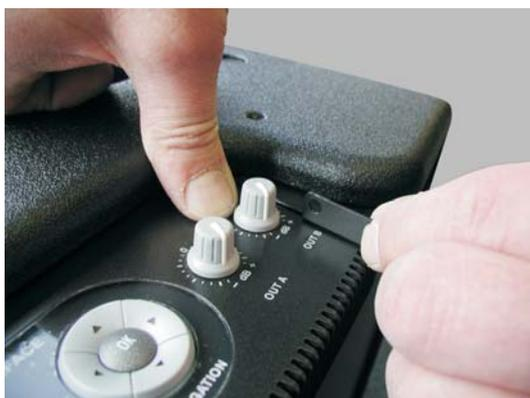
Take the right assembly bracket and slide it between the electronic chassis and the loudspeaker housing as described above.
