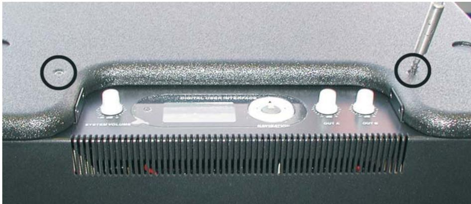
Lay the protective hood on the Navigation board(1.) and snap it in like here(2.).
