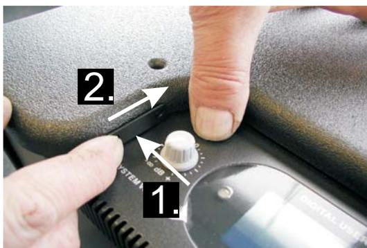
Position the assembly bracket by pushing it up against the side(1.) and the back(2.). Keep pushing the electronic chassis *lightly* while positioning the bracket to move it easier.
