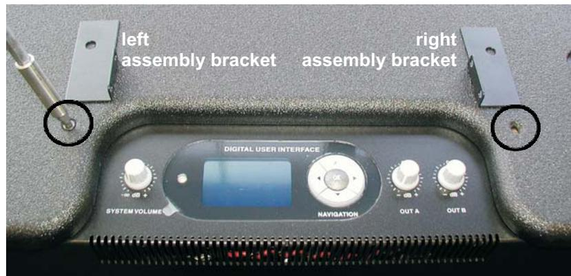
At first, place the left and the right assembly bracket ready and unscrew the two screws at the top of your VSS 15/18 with a screwdriver Torx 20.
