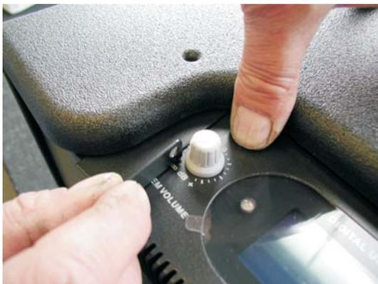
The next step is to push *carefully* with your thumb on the electronic chassis and to take the left assembly bracket. Slide this assembly bracket with your other hand between the chassis and the loudspeaker housing.
