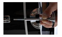
Hand-tighten all eight screws. When doing this, tighten the screws in the diagonally opposite sequence. You only need to tighten the screws slightly, we will be tuning the drums later on.
