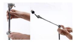
Push the centre and spacer tubes onto the bottom case and fix them with the wing screws. Now push the boom through the joint and fix it temporarily with the wing screw. We will make the final settings later on.
