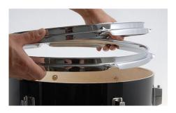
To make the hoops easier to transport, they are fixed on one side of the shell with a couple of screws. To mount the heads, you must first completely remove the hoops. Now lay a head on the shell and put a hoop over it. Both the hoops and heads are exactly the same so it doesn't matter which one you use where. If you look from the top, you can see whether the head and the hoop are really contacting the middle of the drum shell.
