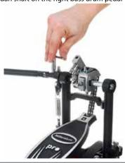
Step 3: Tighten chain on the right bass drum pedal
