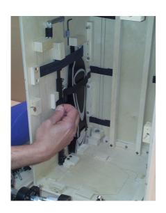
Then remove the transmission bracket.
