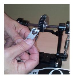
Join the foot platform to the chain post, if you are right footed the post shall be placed at the right side to the foot platform if you are left footed then it's the opposite way.
