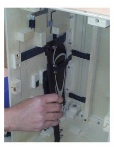
The transmission bracket has compulsory positioning, with the thinner part facing upwards, and the tightening bolts towards the front panel.
