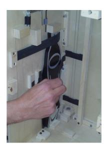
Finally, remove the foot platform.
