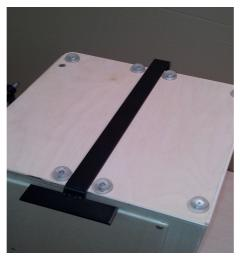
Place the cajon onto the bottom clamp, making sure it is caught between the four rubber guides.
