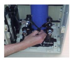
Remove the double sided velcro that unites the beater bar to the pedal chain, which function is to prevent any of those pieces to wander randomly and cause damage inside of the instrument.
