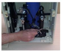
Remove the beater post by unfastening the clamp with the drum key that comes attatched.
