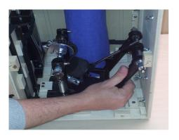
When removing or placing the beater post always keep it at an angle to ease the movement.
