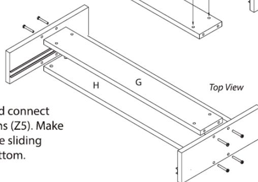
**6.** Align Boards (G & H) to Boards (I) and connect by inserting Bolts (Z1) through the Cams (Z5). Make sure that Board (G) is on the top and the sliding tracks found in Boards (I) are on the bottom.
