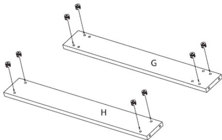
**5.** Place boards (G) and (H) on a flat surface and insert Cams (Z5) into the holes as illustrated.
