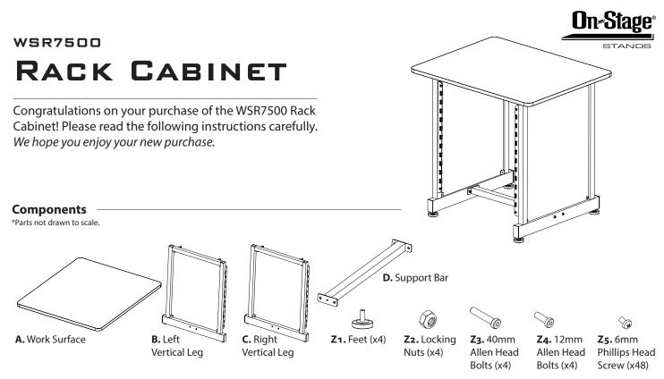
Also included: Allen Wrench Tools Required: Level, Hammer, #2 Phillips Head Screw Driver, & 3/8 Wrench
