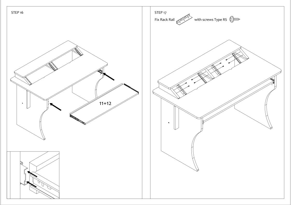
If you don't need the rack units don't fix the rack rails and use the pieces number 13 to close the holes
