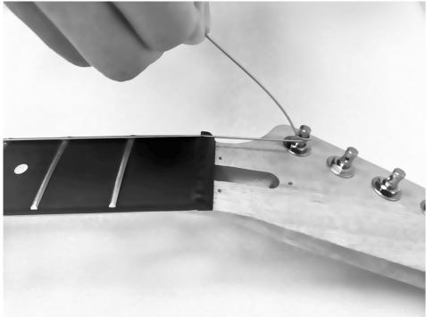
Then tune all the strings in sequence to the correct pitch. You can use a tuner or a pitch pipe as a reference. Note that the string tension will drop a little and the guitar needs to be retuned several times until the strings stay in tune.
