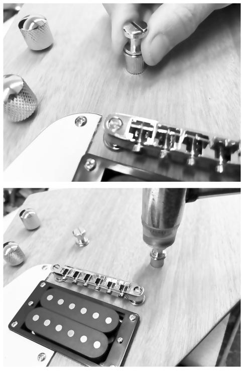
Attach the tailpiece using the screws provided. If necessary, adjust the position of the earthing wire so that the tailpiece can be mounted flat on the guitar body using the fastening screws.
