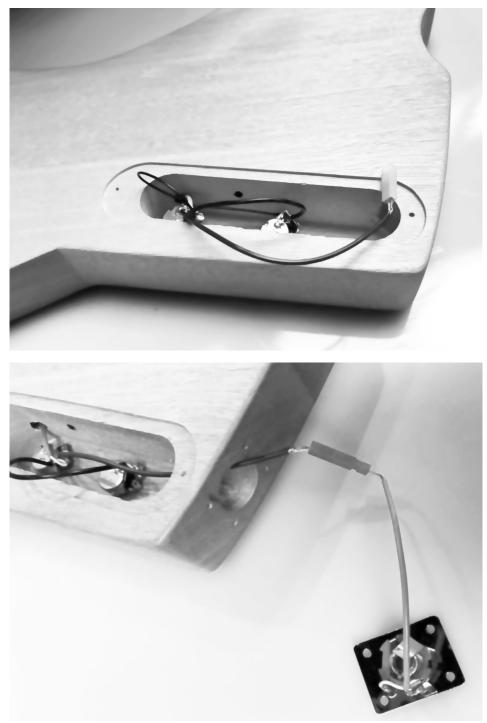
Insert the jack bush into the hole provided on the base of the body for this purpose, and connect the two plug connectors.
