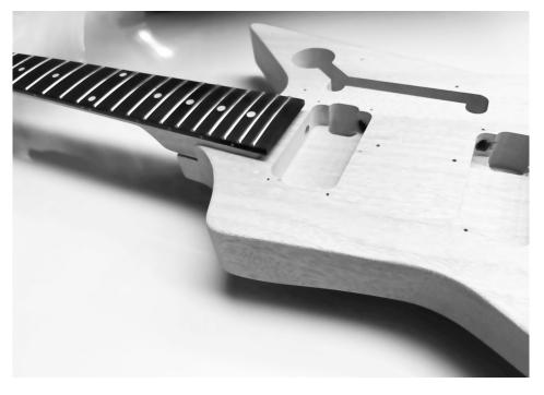
Turn the guitar over, position the mounting plate over the four screw holes on the back of the body and screw the four supplied long wood screws through the holes in the mounting plate into the body and neck until the connection is firm.
