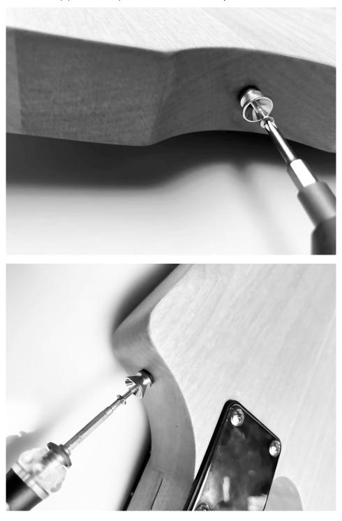
Screw the strap pins into the pre-drilled holes in the body as shown.
