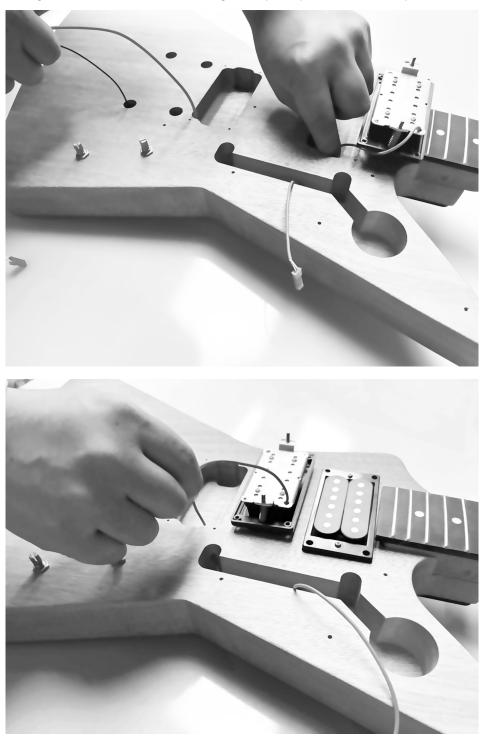
The pick-ups, pots and jack are connected to a cable harness with click-on plugs. Prepare the neck pick-up and the bridge pick-up for installation by routing the cables through the recesses and then screwing in the pick-ups as shown in the photo.
