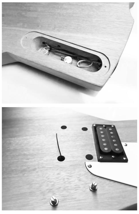
Route the string-earthing cable through the lower cable channel and to the hole for fastening the tailpiece.
