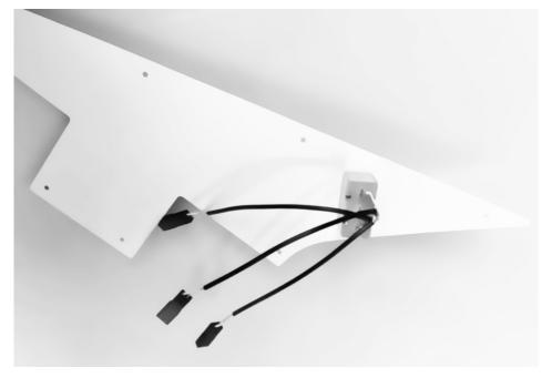
Route the switch from the back of the pickguard into the designated hole and screw it in so it is hand-tight.
