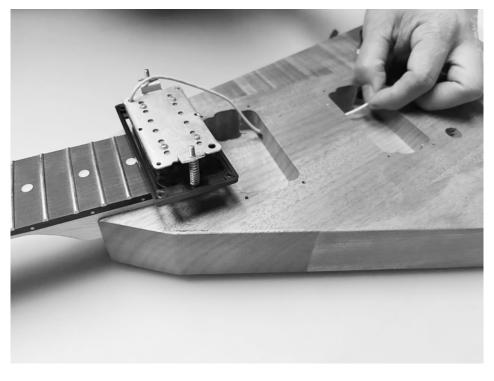
Thread the neck pick-up cable (yellow) as shown in the picture through the cable channel into the recess for the bridge pick-up and from there further through the cable channel into the back recess for the pots.
