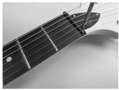
Screw the cover for the truss bar onto the header headstock.
