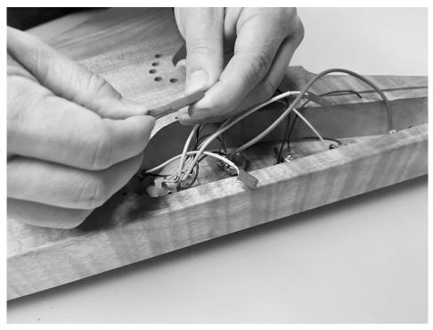
Connect the switch, the pots, and the pick-ups as shown in the picture to the cable harness plug connectors in the back recess.
