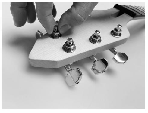
Turn the neck and fasten all the machine heads finger-tight to the front of the headstock with the washers and nuts provided.
