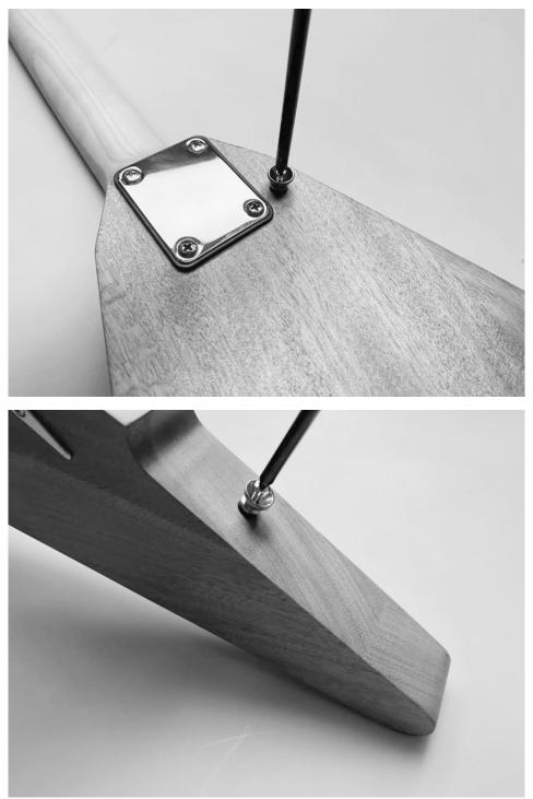
Screw the strap pins with the supplied screws into the pre-drilled holes in the body as shown.
