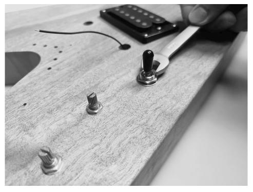
Put the supplied nuts and washers onto the switch, the pots, and the jack socket on the front and tighten the nuts with an appropriate spanner.
