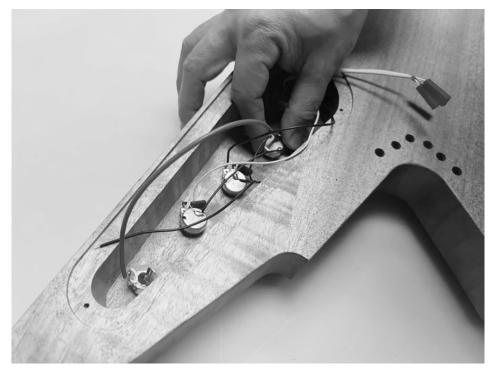
Thread the string-earthing cable from the back recess through the cable channel into the tailpiece mounting hole.
