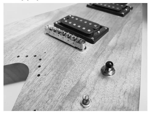
Put the bridge onto the mounting bolts. The bridge is still loose and is only fixed when stringing the guitar.
