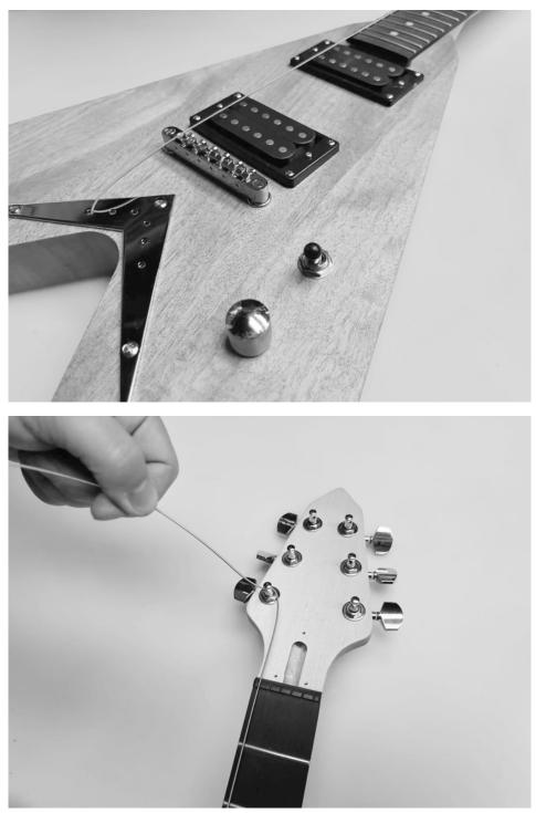
Then tune each string in turn to the correct pitch. You can using a tuner or a pitch pipe as a reference. Please note that the string tension will still drift and the guitar will need to be retuned a few times before the strings are played in.
