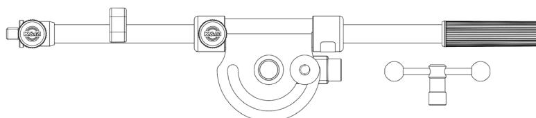
Boom arm with T-bar locking screw
