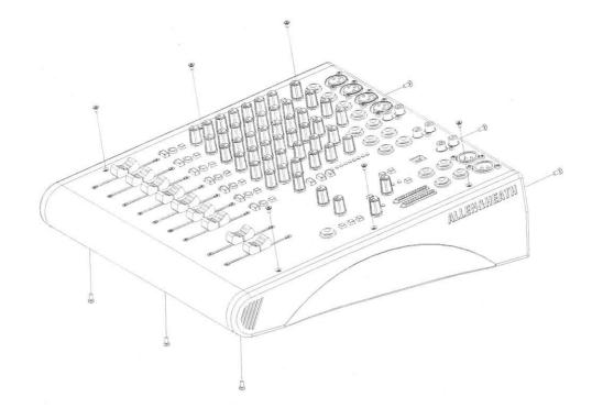
Carefully remove the top panel by gently pulling the back end upwards and sliding the panel forward. Place top panel on left hand side of mixer base. Care must be taken not to pull on connecting power cable.
