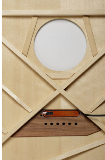
Steel string at bridge plate
