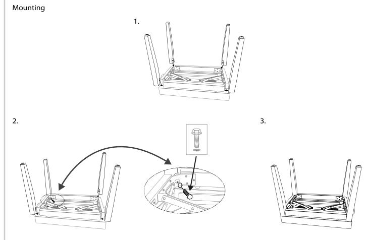
Tighten the screws manually. Put the bench in a stable position on the floor. Tighten the screws only then using the included wrench. This ensures that the bench does not shake.
