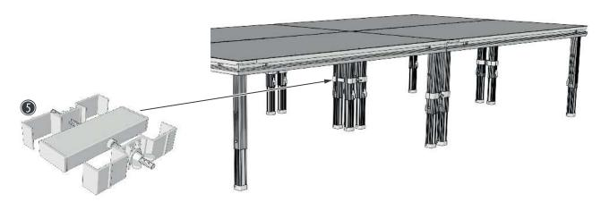
**4.** Secure four neighbouring plug-in feet with a 4-way plug-in foot connector (5) and tighten the wing screws.
