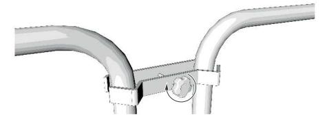
**4.** Secure two neighbouring railings with a connecting clamp and tighten the hand screw. Check the railings for firm fit.
