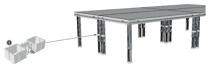
**3.** Secure two neighbouring plug-in feet with a 2-way plug-in foot connector (4) and tighten the wing screws.
