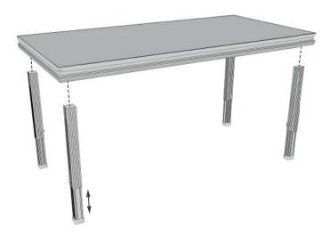
1. Insert the plug-in feet into the designated recess on the bottom of the stage platform.
