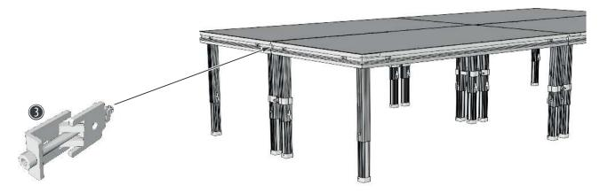
Insert the quick connectors (3) into the profile of the guide rails on the outsides of the stage platforms to be connected and tighten the screws of the quick connectors using an Allen key.
