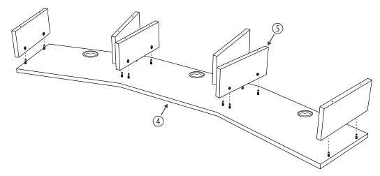
Turn the tabletop over so the bottom is facing up. Place pieces of wood under the drill holes to prevent the coating from cracking out when drilling. Using a 4mm bit, drill the twelve holes through the pre-punched positions on the underside of the table top.
