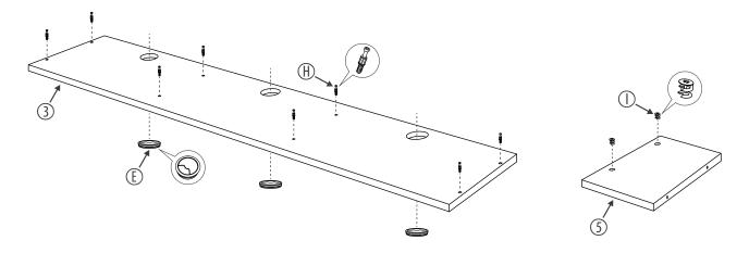
Put the four side panels on the connecting bolts of the monitor bridge and tighten the connector housings of the side panels clockwise to lock the connection with the inserted connecting bolts.
