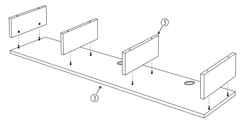
Turn the tabletop over so the bottom is facing up. Place pieces of wood under the drill holes to prevent the coating from cracking out when drilling. Using a 4mm bit, drill the eight holes through the pre-punched positions on the underside of the table top.
