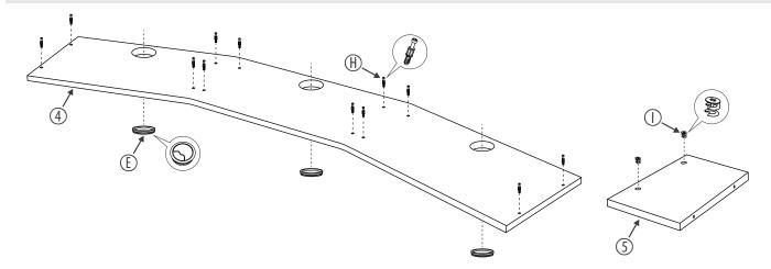
Put the six side panels on the connecting bolts of the monitor bridge and tighten the connector housings of the side panels clockwise to lock the connection with the inserted connecting bolts.
