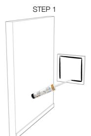
Apply Vicoustic's Flexi Glue at the back of the Multifuser DC2 acoustic panel, near the edges.
