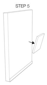
Remove the acoustic panel slightly from the wall surface (approximately 2cm) during 15 seconds.
