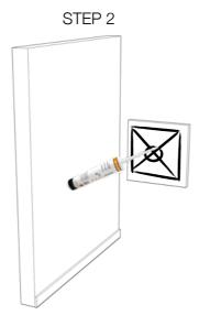
Apply Vicoustic's Flexi Glue in the centre of the Multifuser DC2 like shown on the image above.
