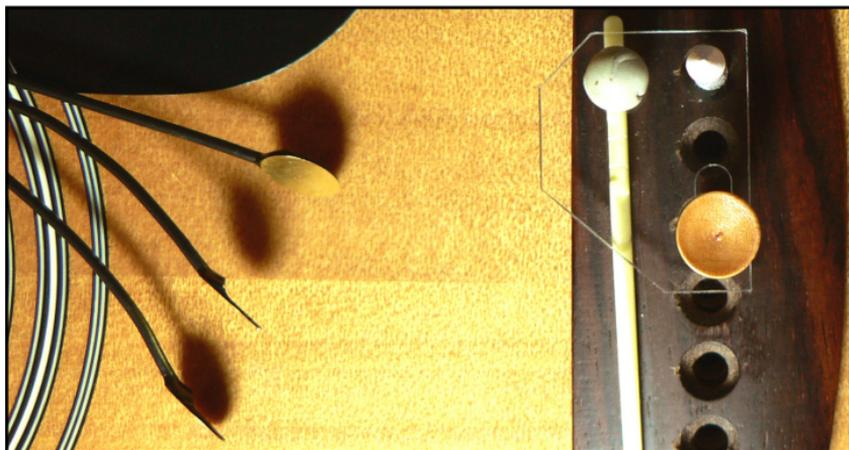
5. Place one pickup on the putty with the golden side facing up and press the pickup to the putty. It should hold the pickup in place securely enough to allow for the installation.
