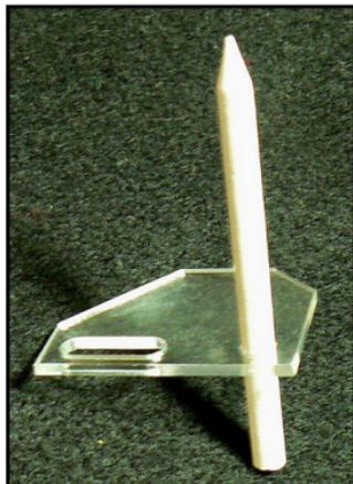
The pin should fit very snugly – you may have to use some force (or even file it down a bit) to press it into the hole. If the pin fits too loosely, please use some superglue to secure it. Wipe off excess glue and let dry.
