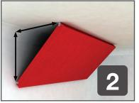
If using a Trap 50L (with square edges), each bracket should be 395mm from the corner.
