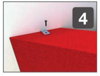
Push your tile between the brackets. Fix 4 suitable screws into the MDF edging of the tile. We recommend using a 'pan head' wood screw.
