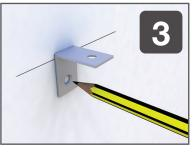
Offer your top brackets up to the lines and mark the holes before drilling and fixing as you did in Step 1. Make sure you position the bracket correctly - the inside of the top leg should be on the line.
