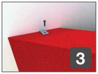
Push your bass trap between the brackets. Fix 4 'pan-head' wood screws into the MDF edging of the trap.
