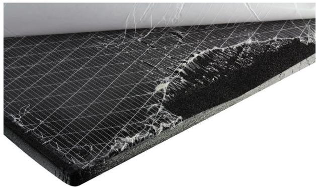
Should the carrier film be removed carelessly or too quickly, the adhesive may stick to the carrier film in some places while being removed from the foam.
