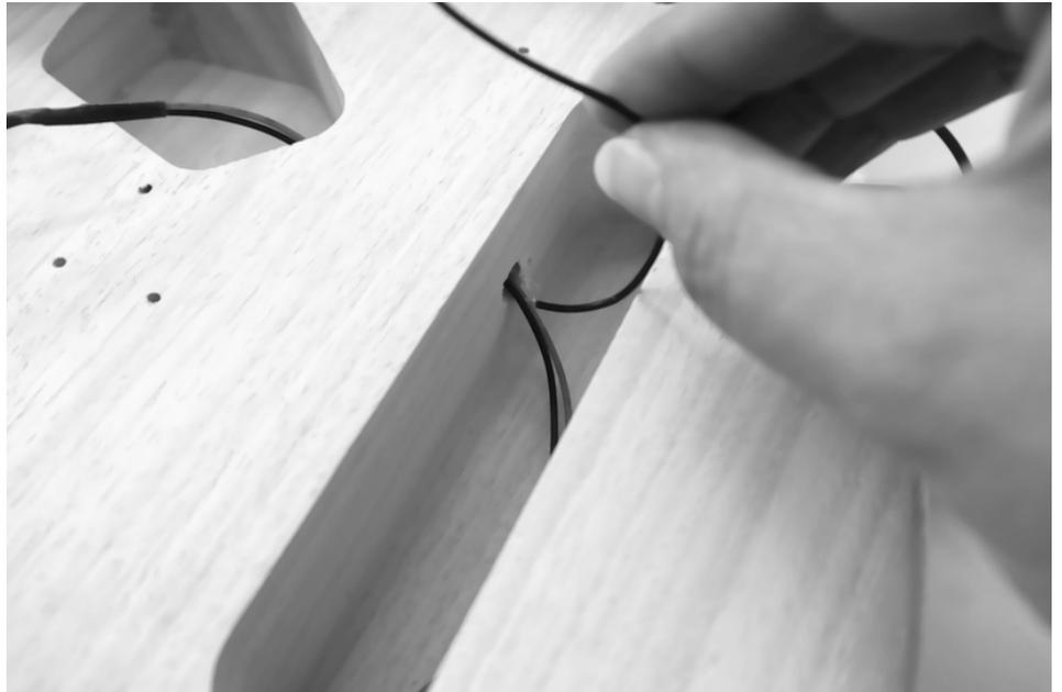
Next, pull the cable out of the hole far enough to ensure sufficient contact with the metallic surface when the bridge is installed. Earthing the strings reduces noise interference.
