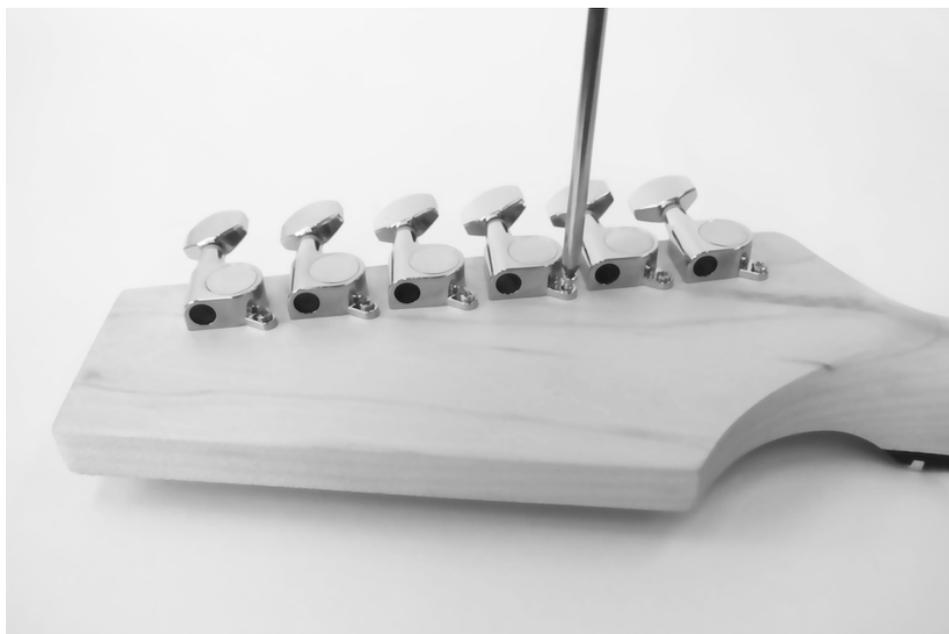
Turn the neck and fasten all the machine heads finger-tight to the front of the headstock with the washers and nuts provided.
