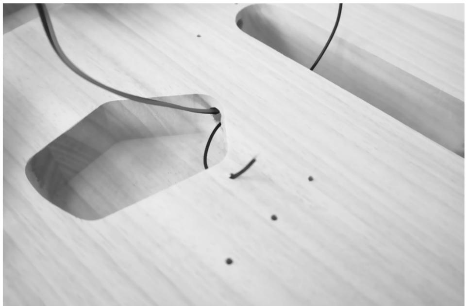
Place the body on a suitable working surface. Use a soft pad in order to avoid damage to the surface. Insert the bridge with the pickup into the cutout on the body as illustrated.
