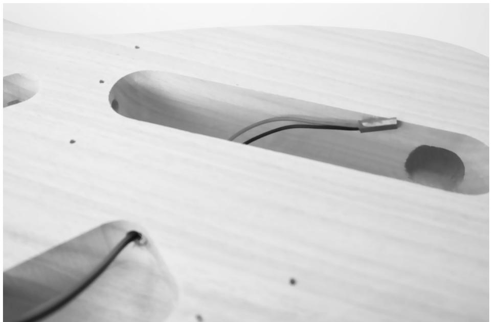
Run the cable for earthing the strings (stripped, without connectors) through the channel in the recess for the potentiometer plate and into the recess for the bridge pickup.
