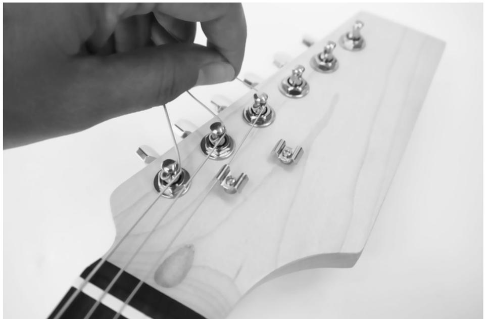
Then tune each string in turn to the correct pitch. You can use a tuner or a pitch pipe as a reference. Please note that the string tension will still drift and the guitar will need to be retuned a few times before the strings are played in.
