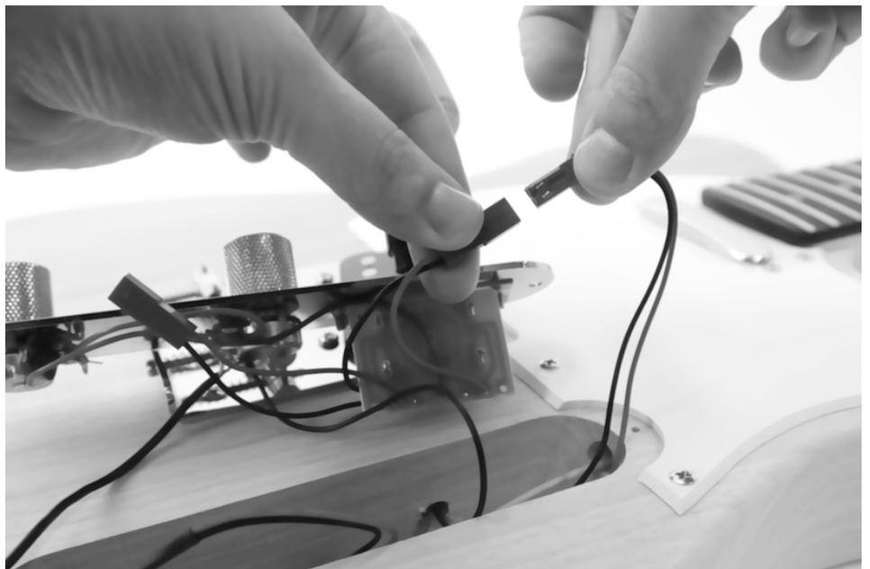
Set the holder for the output jack in place and check whether the jack protrudes. It should stick out over the holder enough that it can be screwed firmly in place with the nut provided, but no further than necessary. Correct the position if necessary by turning the counter nut inside appropriately.
