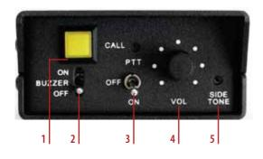
*CALL*-button (1), with light indicator. Below is the buzzer ON/OFF switch (2), to generate an acoustical call buzz. In the middle of the panel is the 3-position microphone switch: *ON* (permanently), *PTT* = Push To Talk and OFF (3). Finally the volume control for the earphone (4) and the *SIDE-TONE-control* (5) for setting the cue volume of your own microphone. For all these controls the same hints apply as outlined for the master station MS-200.
