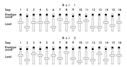
Note that in addition to a level control, each step has an Envelope On/Off switch. If set to OFF, the step level is held constant throughout the entire step; if set to ON, then the sequence's output ramps up from zero to the programmed level value at the start of the step, then immediately ramps back down to zero, as shown below:
