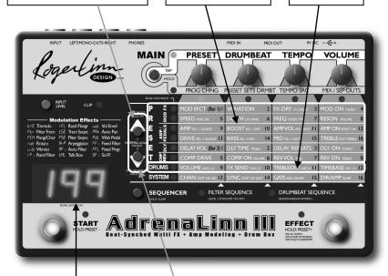
The display shows the value of the parameter at the lit row and column. To select an unlit column without changing any data, turn its knob one 'click'.
