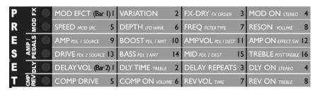
The upper 2 rows contain the Modulation Effect settings, the next 2 rows control the Amp and pedal settings, the 5th row controls the Delay settings and the 6<sup>th</sup> row contains the Compression and Reverb settings. Also note some numbers printed in black. These are the sequence settings, explained further in this chapter.
