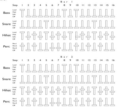
Editing the drumbeat sequence uses an alternate mode of the 8 x 4 parameter matrix in the center of the panel, where the 32 steps printed in gray ("Bar 1, 1-16" and "Bar 2, 1-16") replace the 32 parameter names printed in white:
