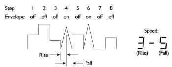
The rate of envelope rise (attack) and fall (decay) depends on the Speed control, which has the format "x-y" ("x" is the attack time of 0 to 9 and "y" is the decay time of 0 to 9).
