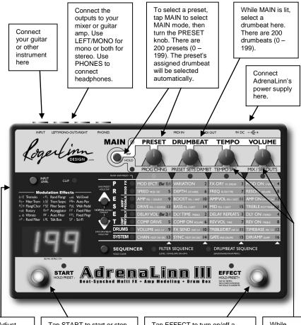
Adjust INPUT LEVEL so that CLIP lights only when you play very hard. Tap START to start or stop the drumbeat. HOLD to decrement the preset. (Tapping START starts the drumbeat on the switch release; to change it to start on the down stroke you must remove the HOLD function. See the end of the Assigning Foot Switches section in Chapter 4.)
