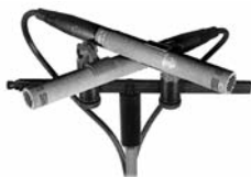
Fig. 2 ORTF , distance between capsules: 17 cm, angle: 110° (green markings)
