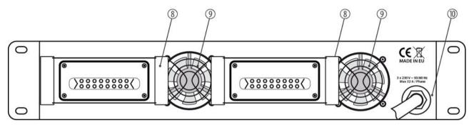
8 Dimmer outputs, 2 × 16-pin Harting industrial connectors (note the device label when connecting the cables).
