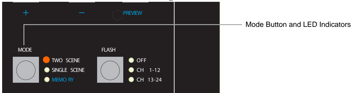
Figure 6: Mode Button LED Indicator - Two Scene
