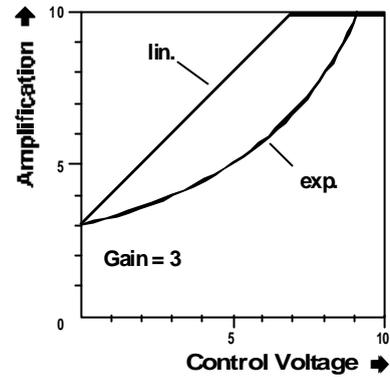
Fig. 2: Effect of gain control on VCA response
