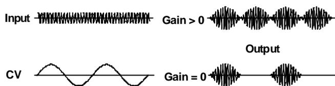
Fig. 3: VCA output level at different gain settings.
