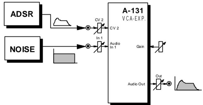
Fig. 4: Time dependent amplification using an ADSR
