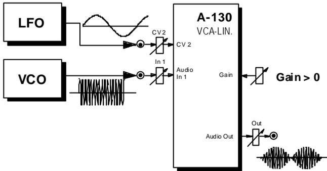
**Fig. 5:** VCA amplitude modulation with an LFO
