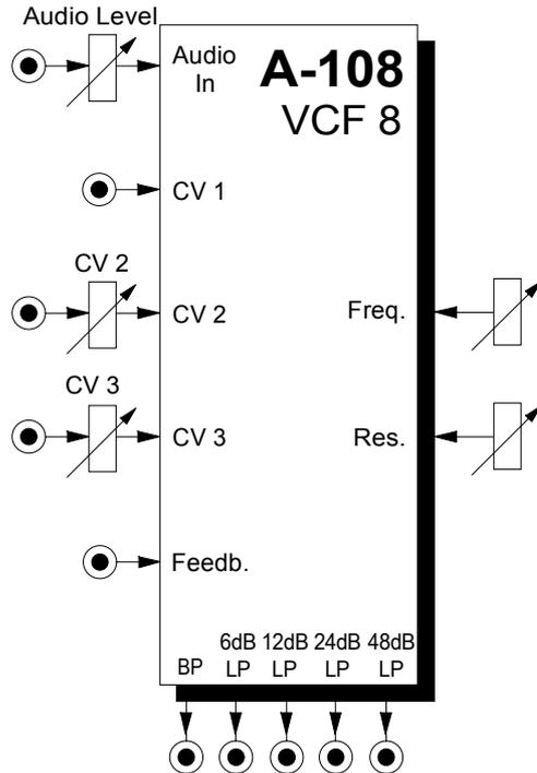
Module A-108 is a completely new, unique voltage-controlled **low pass/band pass filter** based on the well-known **transistor ladder** (Moog ladder).
