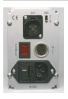
On the back panel of the power supply there are three connectors: power, microphone (Tuchel connector) and signal out (XLR phase signal on pin 2). Additionally there are two switches – power and ground lift – and the voltage setting/fuse holder.
