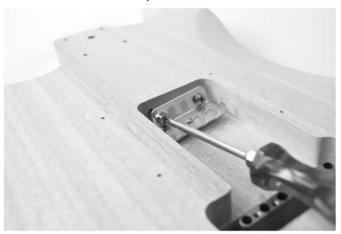
Attach the loops of the three springs to the spring claw and guide the other ends into the small holes in the sustain block. Continue to tighten the spring claw towards the neck until some tension is applied to the bridge.
