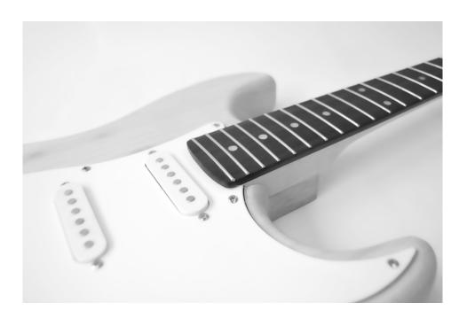
Turn the guitar over and position the neck plate over the four bolt holes at the rear of the body, then screw the four wood screws provided through the neck plate, body and pilot holes in the neck until everything fits tightly.
