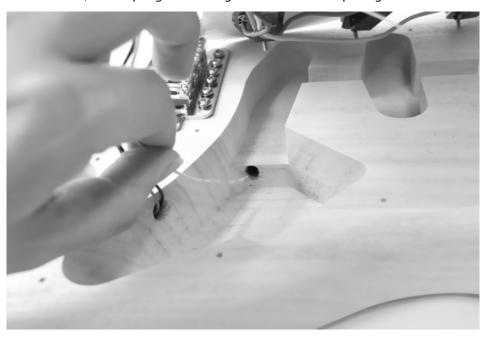
Hook the grounding cable onto the spring claw. Ensure there is sufficient contact between the stripped end of the earthing wire and the spring claw.
