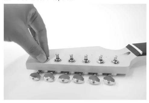
Tighten the nuts on the front with an appropriate spanner, then tighten the screws on the back firmly to fasten the tuners.
