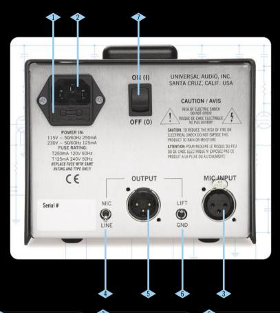
FUSE — IMPORTANT! The SOLO/610 requires a fuse change in the event that the unit will move from 110V usage to 220V usage or vice versa. (250mA for 110V, 125mA for 220) In addition, a jumper most be moved internally (see uaudio.com/solo).
