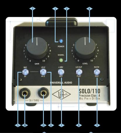
**POWER** – blue LED illuminated when SOLO is powered on
