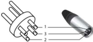
XLR mounting sockets are provided for signal inputs. XLR mounting plugs are provided for signal outputs. Drawings and descriptions explain the pin assignment.
