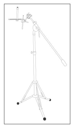
2. Fix the stand clamp assembly in place on the neck of your microphone stand a few inches below the point where the shock mount is usually fixed, or on the main vertical support strut of the stand.
