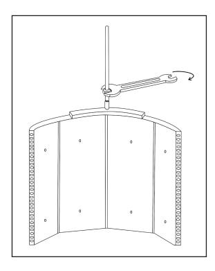
3. Fix the support rod to the Reflexion Filter by screwing it into the socket on the bottom edge. Tighten the nut using the spanner supplied in the box.
