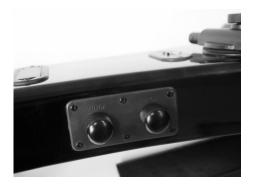
The rotary controls to adjust the volume [VOLUME] and the tone [TONE] (treble, bass) are located at the side of the instrument.
