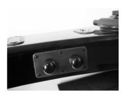
The rotary controls to adjust the volume [VOLUME] and the tone [TONE] (treble, bass) are located at the side of the instrument.
