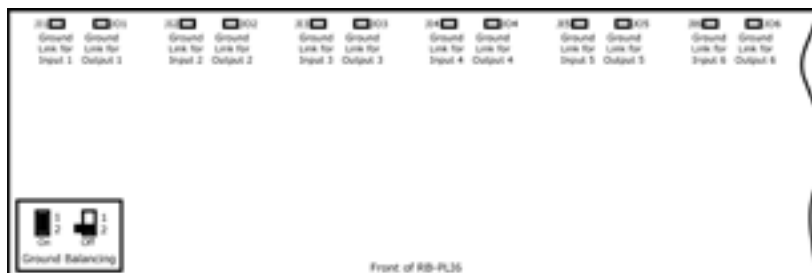
Fig 6-4: RB-PL16 Ground-link Jumper Settings.
