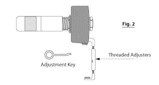
**4.1 Non-permanent external clamp/jack installation:** Open the jaws of the clamp until it fits comfortably over the side of the instrument by turning the threaded adjusters counter clockwise (*See fig. 2*). Set the jack/clamp in place with the protective cork pads completely covering the
