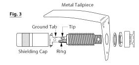
**4.3 Permanent tailpiece jack installation for standard or common style mandolin tailpieces:** First remove the jack from the clamping hardware and de-solder the pickup. Also remove the shielding cap, flat and star washers, and nut from the large threaded section of the jack. You will only need the single flat washer and nut from the small end of the jack for this option. *Note: there is a 1 meg ohm resistor*
