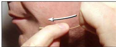
5. Pinch and hold the EarSet boom with one hand and curve it with the other thumb and forefinger to make small adjustments and position the microphone near the corner of the mouth. You may also use the same gentle bending motion to make small adjustments to the other side of the EarClip where it rests over the ear.
