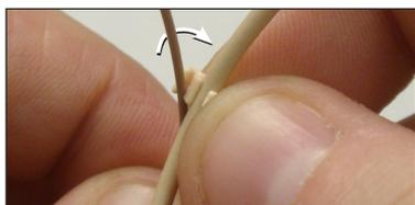
The EarClip cable hook is designed to grip the EarClip and cable very firmly to prevent accidental movement or removal. To remove the cable hook from the EarClip, or to remove the cable from the cable hook, gently twist as shown.
