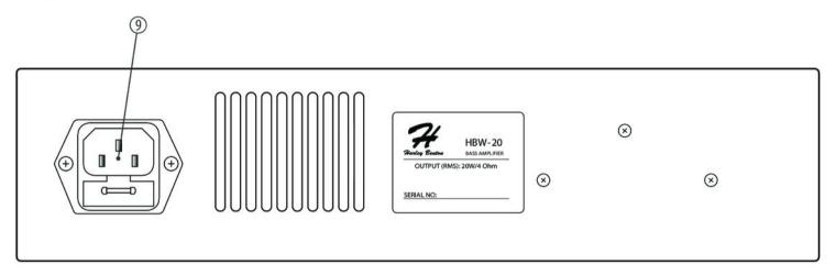
9 Panel plug for mains cable with fuse holder.
