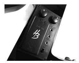
Replace the inserted battery if necessary (weak output signal) or at regular intervals.
