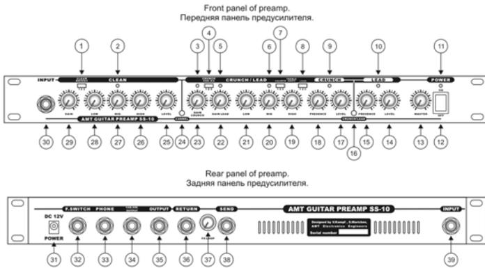
1. Signal correction switch for **CLEAN** channel.
