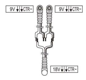
The diagram below shows the cable for supplying the effects requiring 18V DC with polarity CTR + (centre positive) (two 9V CTR - inputs, 18V CTR + output).
