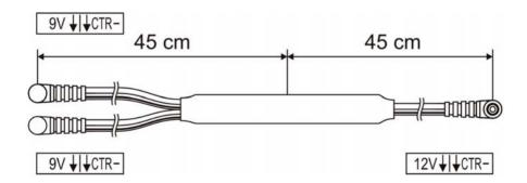
For the effects that require 15V DC voltage it is needed to use individually bought Adapter 2x9V/15V DC (CTR pos. 0,35A) - product code 00866
