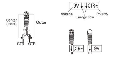
For the effects that require 12V DC voltage it is needed to use individually bought Adapter 2x9V/12V DC (CTR neg. 0,35A) - product code 00865.
