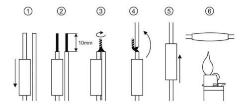
The diagram below shows the way of linking three cables.
