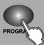
9. If you don't intend to continue your programming, press and hold down the Program button for three seconds to exit Program mode, the LED goes out indicating this selection.
