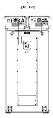
In the first example, a speaker cable with 1/4" or Speakon® ends connects from the speaker output of the amplifier to the speaker input of the Ampeg Heritage SVT-810E cabinet.
