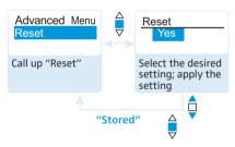
When resetting the settings made in the operating menu, only the selected settings for the pilot tone and for the frequency banks "U1" to "U6" remain unchanged. For an overview of the factory-preset default settings, refer to the enclosed frequency information sheet.
