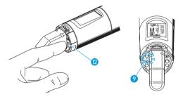
To switch the radio microphone on (online operation):
