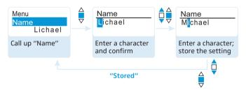
Via the "Name" menu item, you can enter a freely selectable name (e.g. the name of the performer) for the radio microphone.
