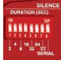
Fig 10-4: SILENCE Detect Duration DIPSwitch
