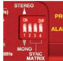
Fig 10-6: SILENCE Detect Stereo/Mono & Sync Source DIPSwitch
