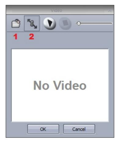
Note that not all AVI compression formats can be read by the software, so your video may need to be converted using media encoding software.
