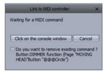
One command on the controller can be used to activate a variety of different commands within the software. For example, you could assign a dial to automatically control the speed of several movement buttons.
