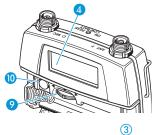
► When switching on the transmitter, keep the ON/ OFF button 10 pressed.
