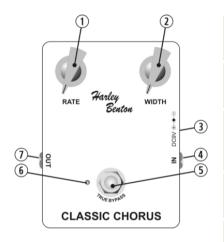
1 **RATE**Turn this knob clockwise to increase the speed of the effect.
