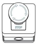
Connect the external safety switch (not included in scope of delivery) to the connection socket provided on the unit. If you press the switch, the laser beam will be switched off immediately.
