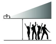
When installing the unit, observe the specified minimum height to prevent the risk of injury to persons, and observe the limits for maximum exposure of eyes or skin to a laser.
