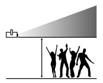
In order to meet the limits for maximum irradiation (MZB limit value for the non-hazardous irradiation of the eye or the skin with a laser), the device must be installed at a height of at least 2.7 m according to the DGUV V11 valid in Germany.
